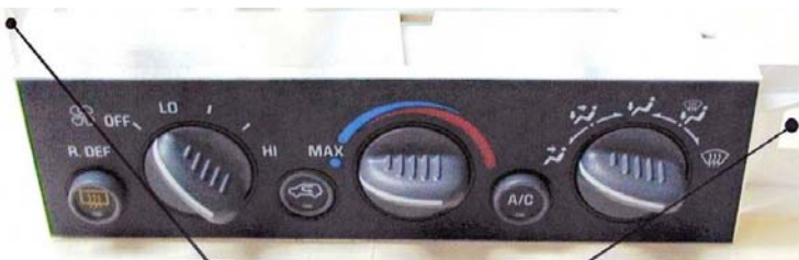
Photo 1. Clips holding in the Control Head
