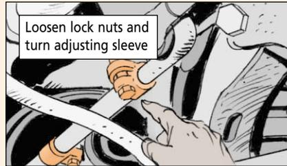
Loosen lock nuts and turn adjusting sleeve
